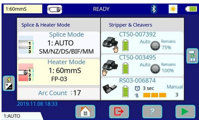
\*Basic operations can be performed from the touch screen after the power is turned on.
