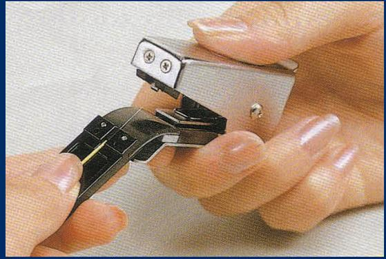
Bending the leaf spring to break the fibre end.
