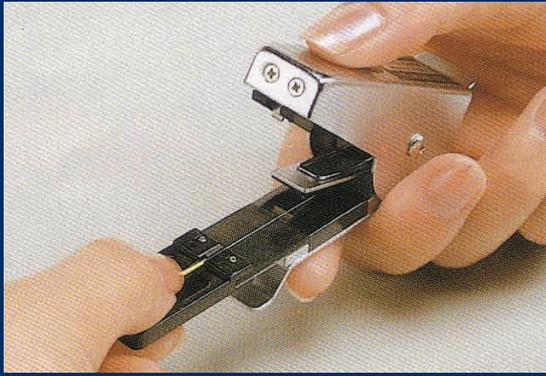
Setting the prepared bare fibre end between the fibre clamp and the leaf spring.
