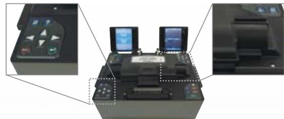
Zero degree fiber holder position – For splicing LDF fibers with minimal core angle, the fiber holders are horizontally positioned relative to the v-grooves.
